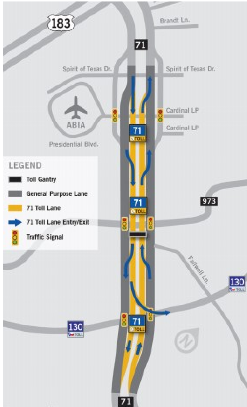
Figure 2-7: 71 Toll Lane Project Configuration
